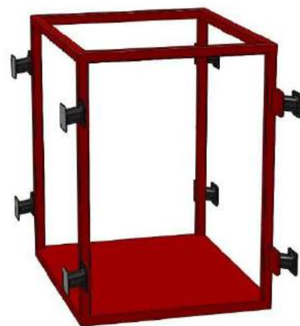
The base of a tower application with a high centre of gravity. Mounts are 'leaning into' the vertical load.
