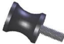
Waisted bobbin – larger impact area to spread force over a larger area and a waist to slow impact over a greater distance.
