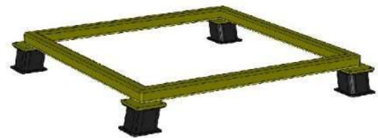
The base of a generator, where mounts were added in pairs facing each other.
